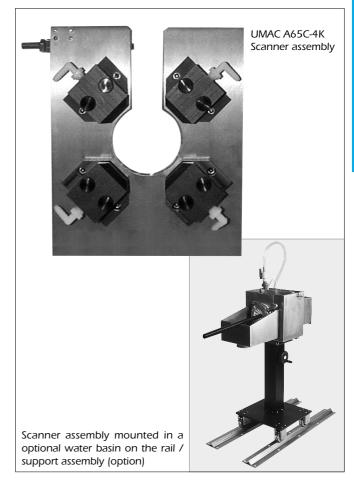
The four measuring points are oriented 90 angular degrees from each other with a 45 degree offset from the vertical and horizontal plane, corresponding to the location of most extruder centering screws.
