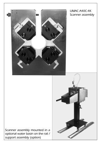
The four measuring points are oriented 90 angular degrees from each other with a 45 degree offset from the vertical and horizontal plane, corresponding to the location of most extruder centering screws.
