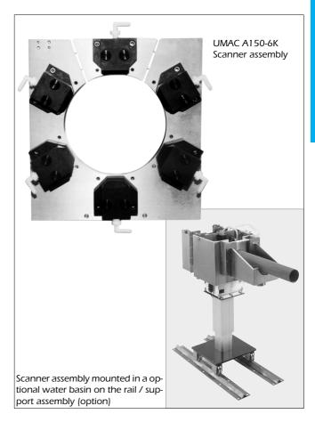
The six measuring points, are oriented 60 angular degrees from each other. Two are mounted into vertical axis and four 60 degrees to the vertical axis. The U-frame construction with removable top section allows for quick removal of product, ready to be mounted into an existing cooling trough or optional water basin.
